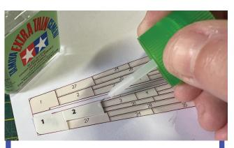
Take plate 2 and glue the 1mm overlap onto plate 1. The faint line shows where this plate should end.
