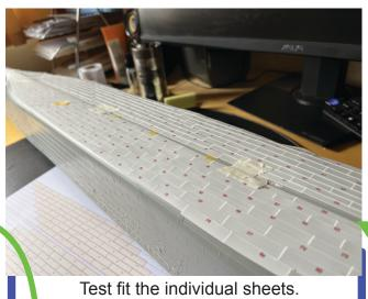
Test fit the individual sheets. You start aft and work forwards. The edge of these sheets should perfectly line up with this edge along the hull.
