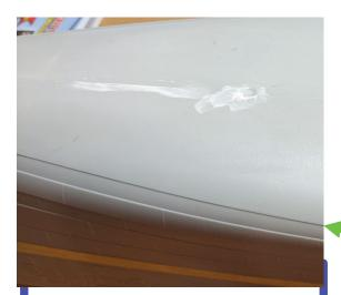
Prepare the kit hull. Sand flush or fill and mould points along the keel.
