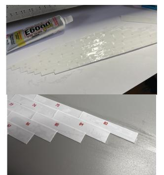
Tamiya Model cement works by melting the plastics together. It was much cleaner to use and none oozed to the surface. It needs to be applied in smaller stages due to a faster drying time.
