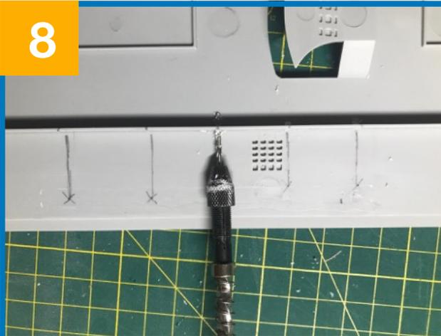
Drill through the LED strip wall with a 1mm drill bitt.
