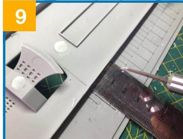
Using the 1mm Scribing tool and a metal ruler, cut channel along your marked lines
