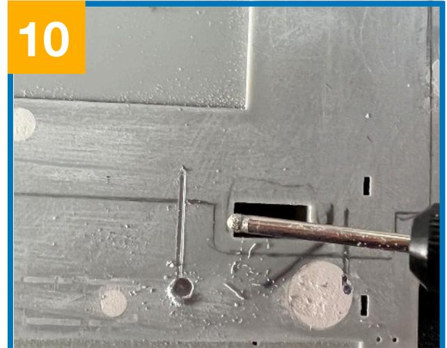
To provide finer adjustment of the light output location, you may want to use the Rotary tool to make a wider hole.
