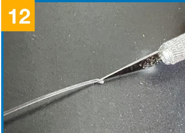
With a sharp blade, trim the end to the correct length.
