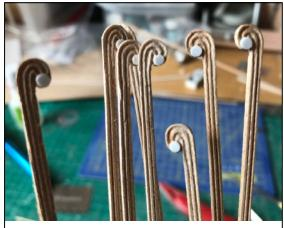
**STEP 7:** Using 0.5mm thick styrene, cut out small circles and glue in place.
